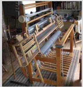
Jack Lane's handmade 45 inch eight shaft loom.
