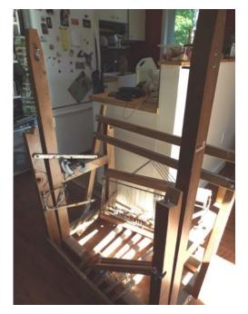
So now the loom was put back together, refinished with Danish oil, and it looked amazing. Then: I tied up treadles one and six for tabby, treadles two, three, four and five for twill, and tried treadling. Treadles two and four worked as they should. All the others pulled down the correct harnesses – but the harnesses wouldn't return to neutral when the treadle was released.
